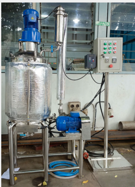
Lithium Carbonate Precipitation Reactor
